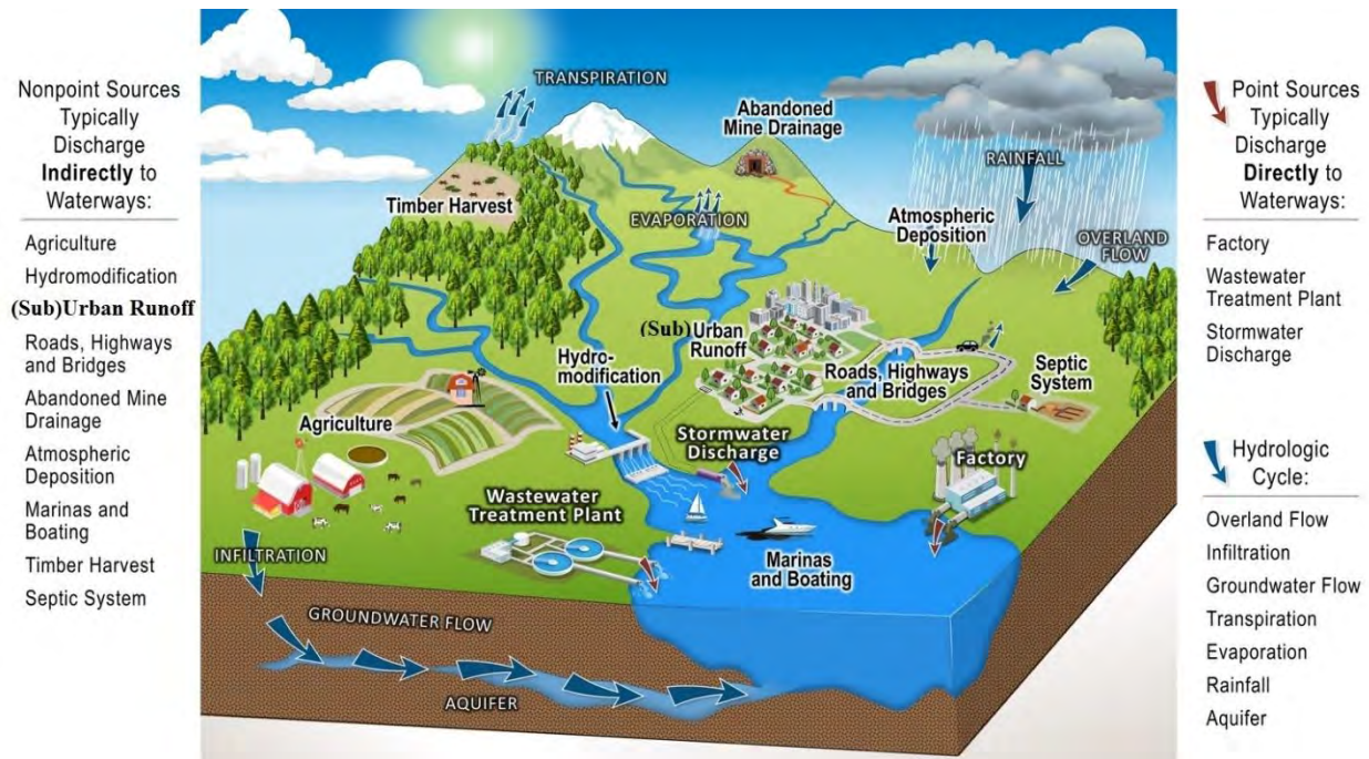
Non-point and point source pollution along with elements of the water cycle
